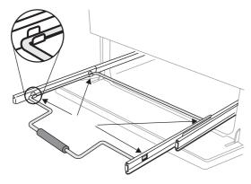
For each side, support the side rail with one hand and with the other hand lift the frame up and out of the side clips.
